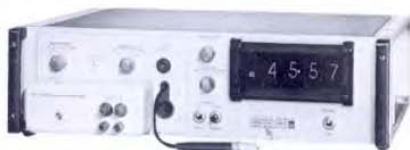
Figure 9. The 1820-P3 Dc Differential Adaptor, shown in place on the 1820-P2.
